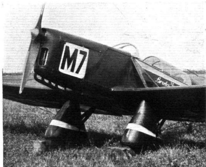
**MISS SPOONER'S "BREDA 33":** The wheels are carefully faired in, and have a travel of nearly one foot (including the deflection on the tyres). The slots extend over the whole wing span. The engine is a de Havilland "Gipsy III."
