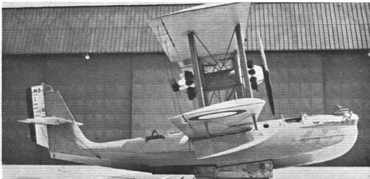
**THE C.A.M.S. (S.G.A.) 55 :** The hull is of all-metal construction, with Duralumin planking
