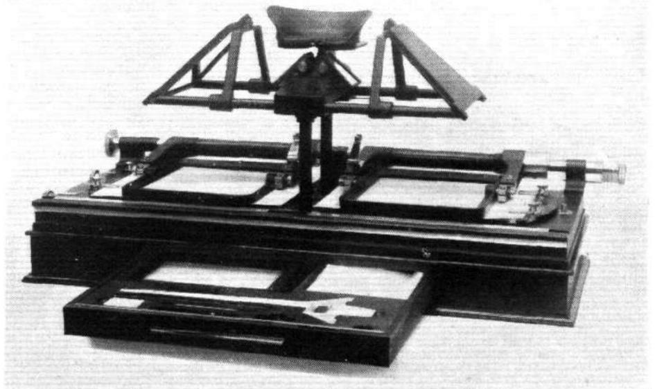
The Barr and Stroud Topographical Stereoscope Type Z.D.10.
