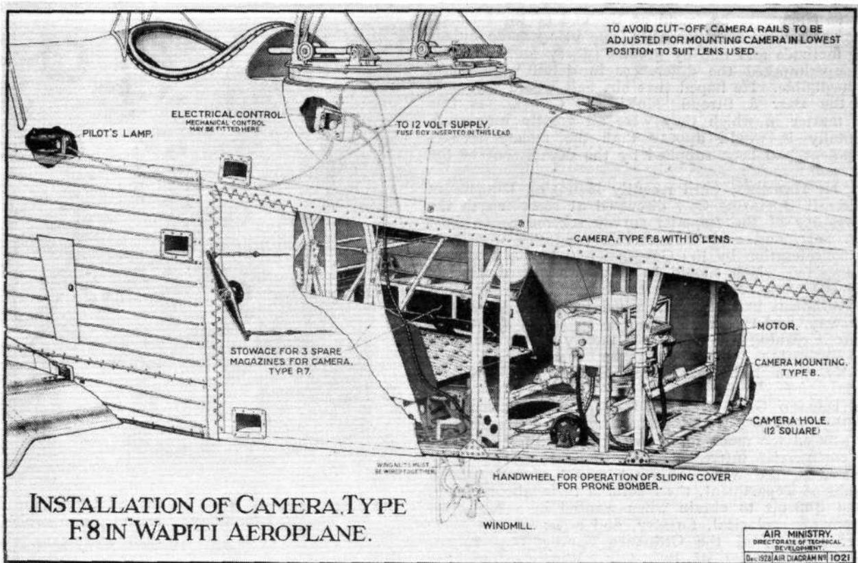
**INSTALLATION OF CAMERA TYPE F.8 IN WAPITI AEROPLANE.**
