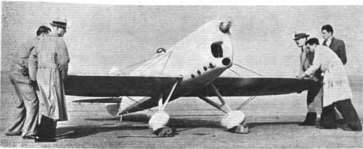
**TO BREAK THE CAUDRON RECORD:** A small high-speed low-wing monoplane, designed and built by Larry Brown, of Santa Monica, California, to attack world's records in its class. It is fitted with a 185 h.p. "Menasco" 4 cyl.-in line air-cooled engine, and is claimed to have a speed round about 240 m.p.h.
