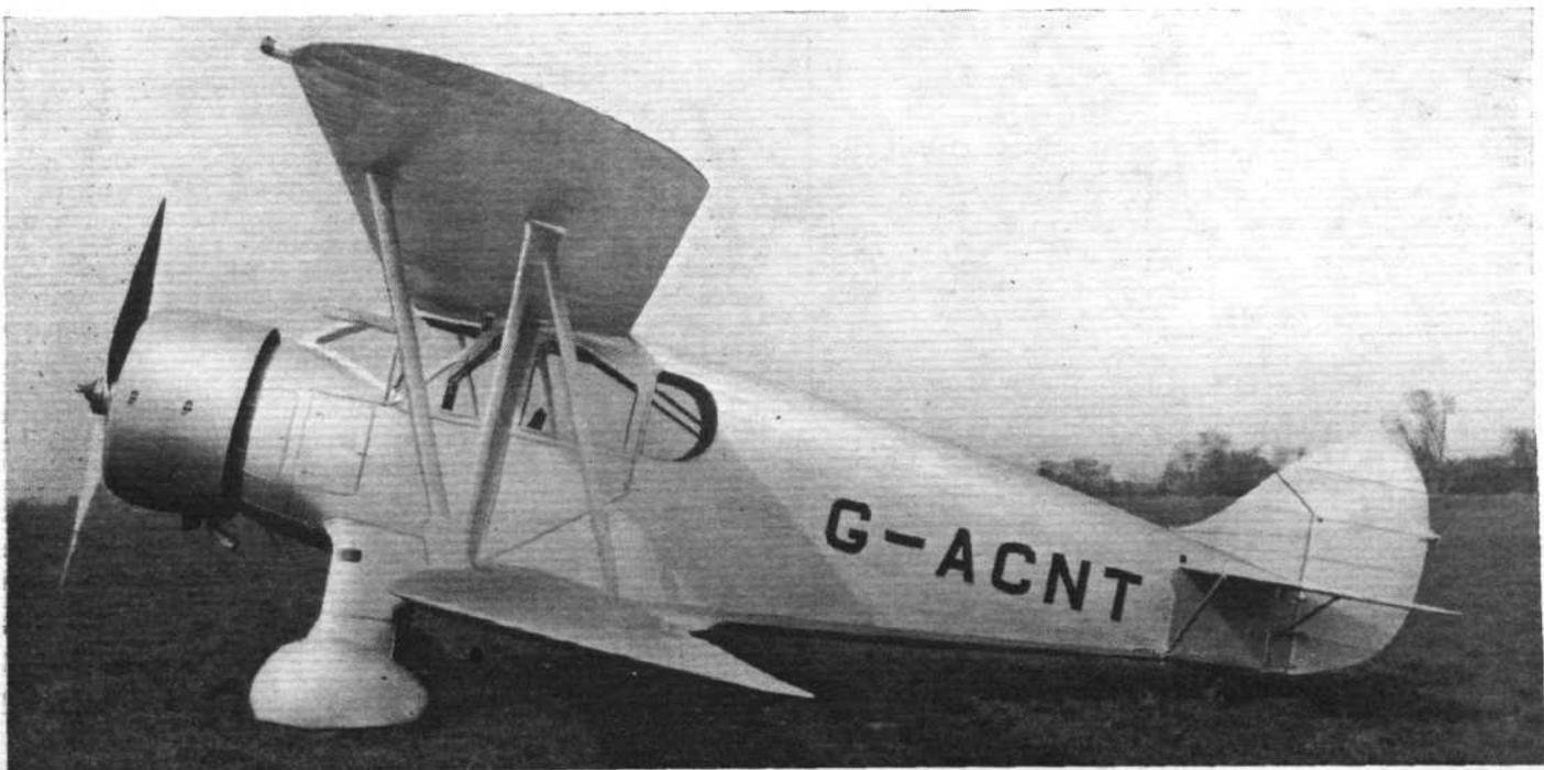
**FOR COMFORT AND SOLIDITY:** Spectacular performance has not been sought in the design of this "Lynx"-engined Avro. The machine is a 4-5 seater with dual control, and is finished and upholstered in a style comparable with that of a high-class motor car.
