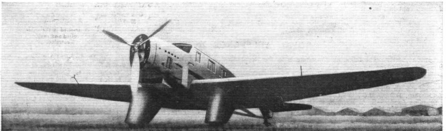
**THE LATEST WIBAULT:** This Wibault 366 carries five passengers, or the mail equivalent, at a cruising speed, it is reported, of 190 m.p.h. It is of particular interest, if only because the engine, an Hispano-Suiza, 12 Ybr. (860 h.p.), is water-cooled—which is rare in a commercial machine to-day.
