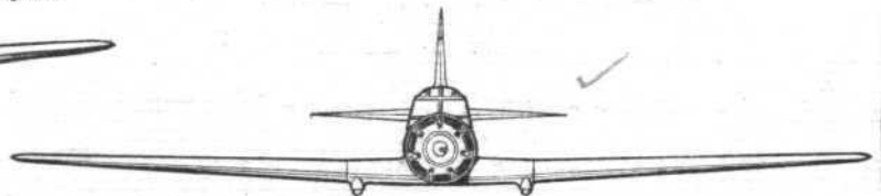
32. 53. S. & H. Lockheed Orion. 550 h.p. Pratt & Whitney Wasp 51D1. Gross wt. 7,750 lb. Wing Area 262 sq. ft. Fuel 500 gallons.
