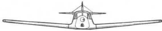
1. H. B.F.W. ME-108 230 h.p. Hirth H.M.18a Gross wt. 2,580 lb. Wing Area 143 sq. ft. Fuel 63.3 gallons.
