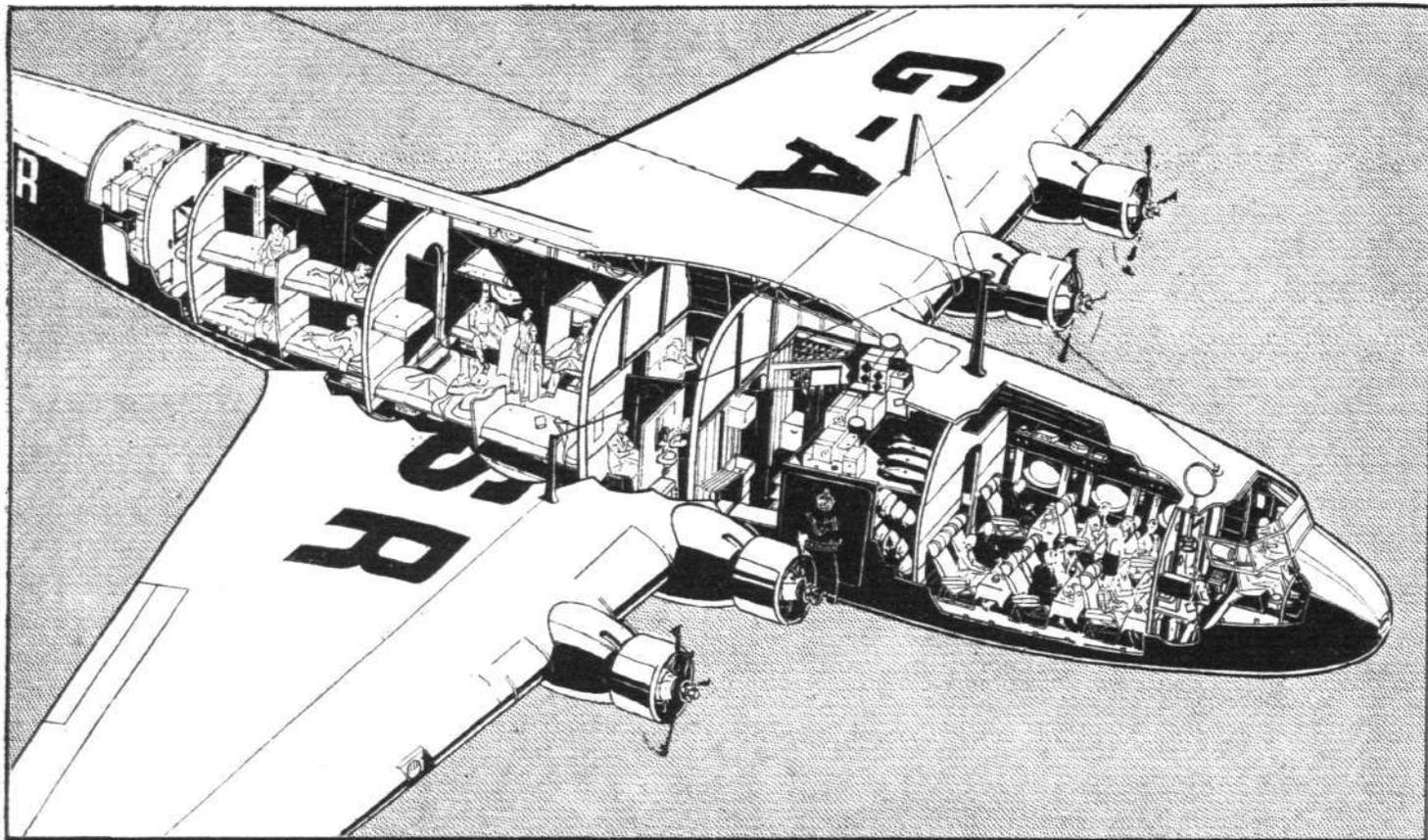
An idea of the spaciousness of the internal accommodation of the A.W.27 machines for Imperial Airways is given by this cut-away drawing.
