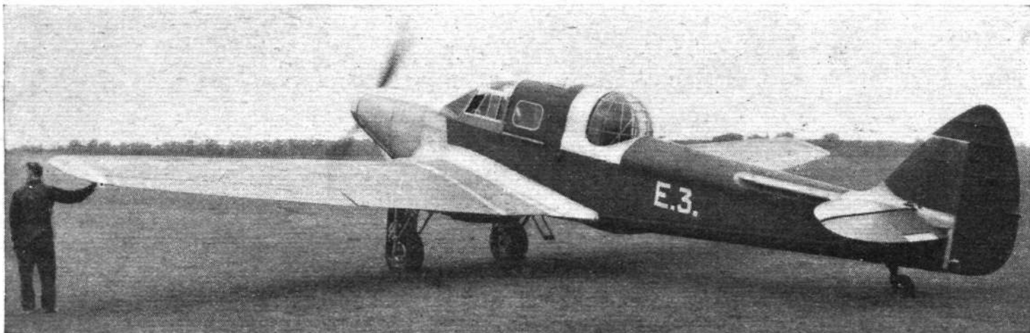
The De Havilland Don advanced trainer, ordered in quantity for the R.A.F., is fitted with the D.H. Gipsyking inverted vee-twelve engine, better known as the Gipsy Twelve. ( Flight photograph.)
