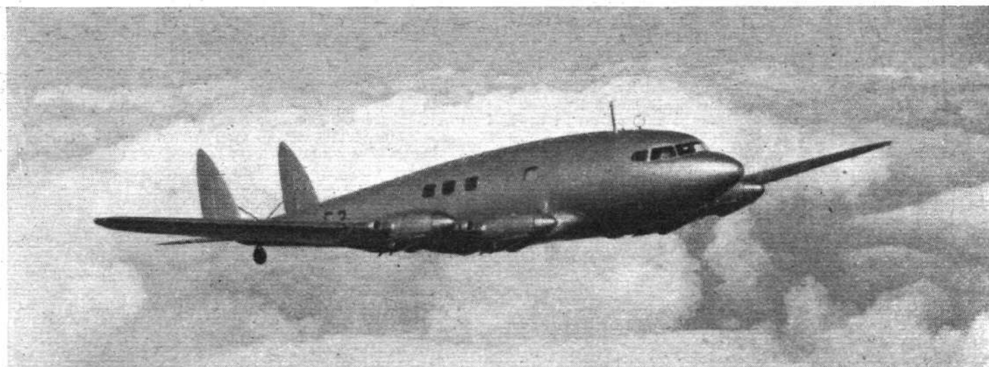
One of the most impressive transport aeroplanes ever built, the De Havilland Albatross is estimated to cruise at about 200 m.p.h. Its four engines are Gipsy Twelves. ( Flight photograph.)
