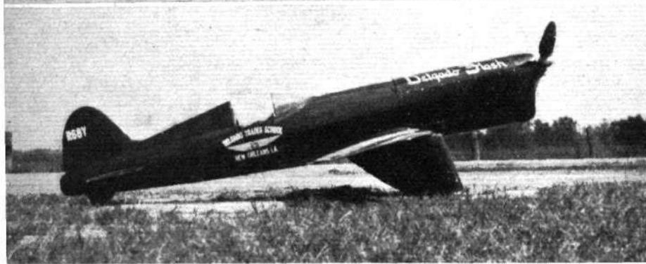
C. H. Gotch's Keith-Rider Special (top) and the Delgado, both of which have small Menasco in-line engines. The Delgado, built by students, is comparable with our T.K.4.
