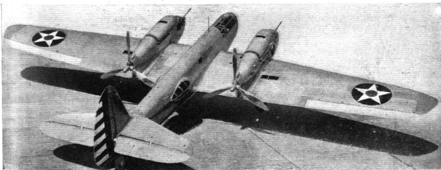
UNORTHODOX: Two illuminating new views of the American Bell Airacuda ("Tiger of the Sky") pusher multi-seater fighter fitted with two 1,000 h.p. Allison liquid-cooled engines with exhaust-driven superchargers. Two "cannons" are mounted in the nacelles and there are Browning machine guns in fuselage "blisters." The prototype machine is now on test.
