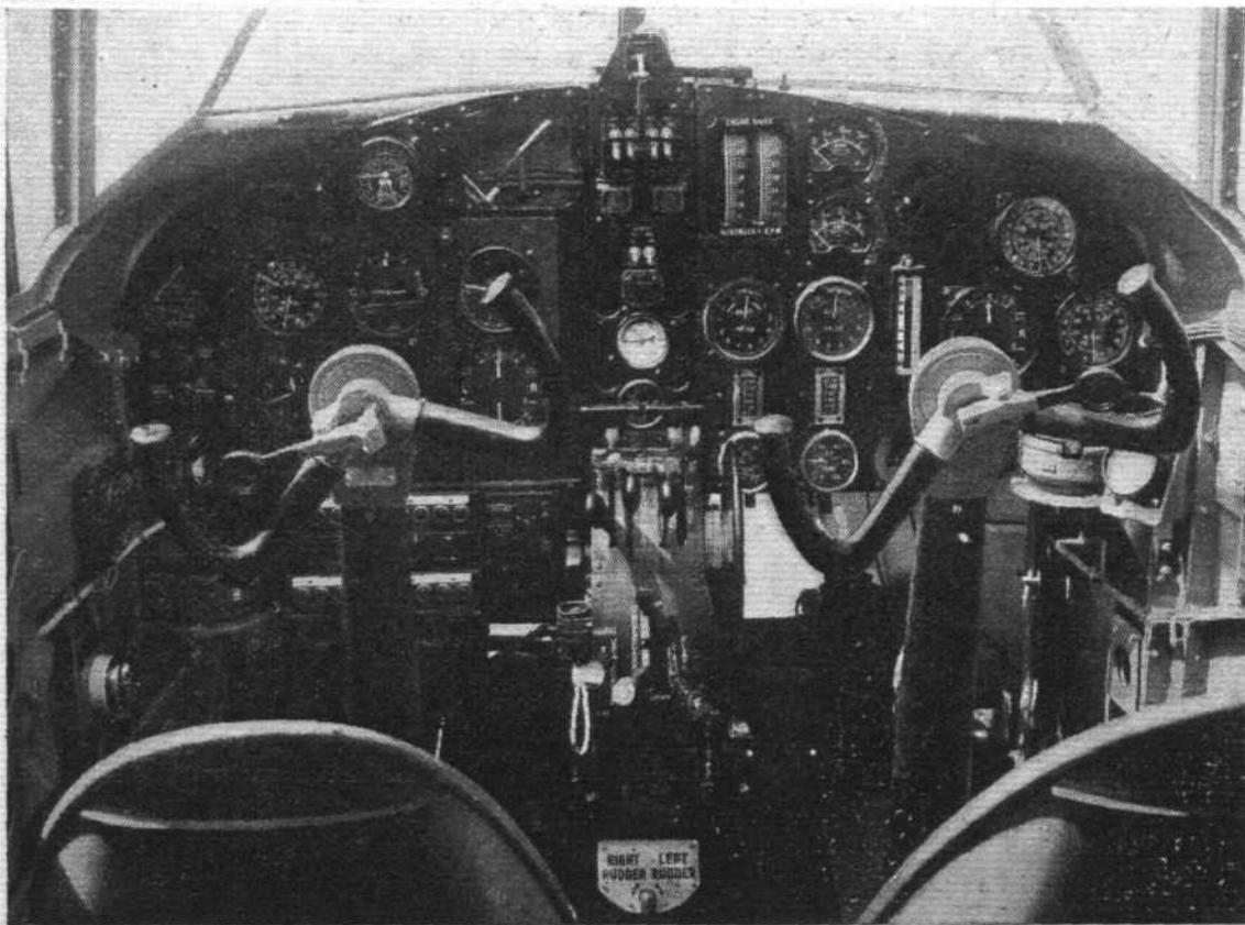
The controls and instrument panel of the Oxford. Below the standard R.A.F.-type blind-flying panel will be seen the bomb release switches. The throttle column carries, also, undercarriage, airscrew pitch and flap controls, together with rudder-bias adjustment. Brake controls will be seen on each control column. A photograph of the instrument board of the prototype Oxford, with the nature of each fitting indicated, appeared on page 603 of *Flight* for June 16.
