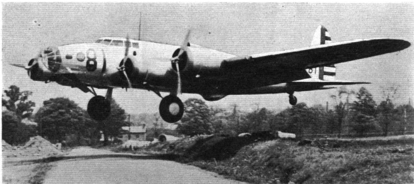
An impressive close-up of one of the U.S. Army Corps Boeing B-17 bombers (two-speed supercharged Wright Cyclones) about to touch down. This machine is considerably smaller than the XB-15 illustrated on a previous page.
