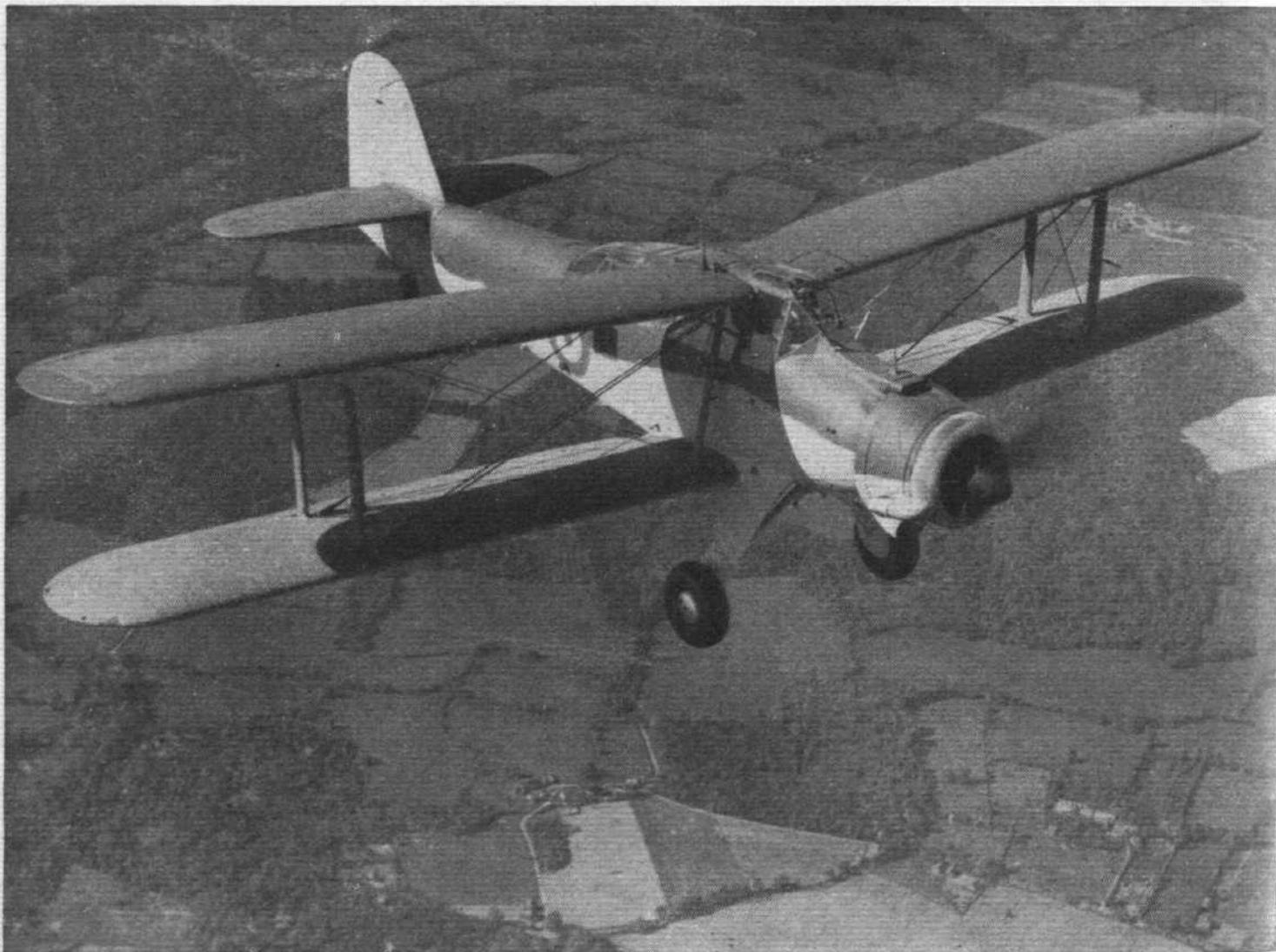
**FOR GENERAL PURPOSES AT SEA:** The Fairey Albacore (Bristol Taurus sleeve-valve engine) which can carry a heavy torpedo, make dive or level bombing attacks, or reconnoitre for the Fleet.
