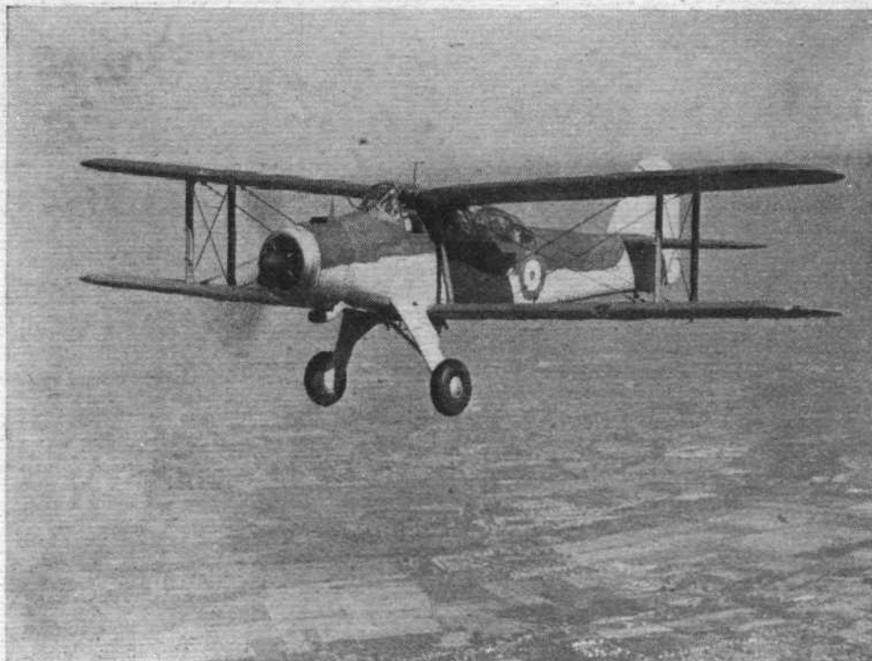
VERSATILITY FOR THE NAVY: The Fairey Albacore biplane which is now in service with the Fleet Air Arm. This machine can be employed for torpedo-dropping, all types of bombing and reconnaissance. The engine is a Bristol Taurus 14-cylinder sleeve-valve unit of over 1,000 h.p.; the small diameter of this power unit enhances the view from the pilot's cockpit.
