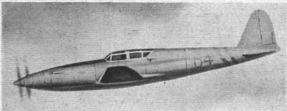
In the A.T.27 the pilot sits between two steam-cooled V-12 engines of 1,250 h.p. each.
