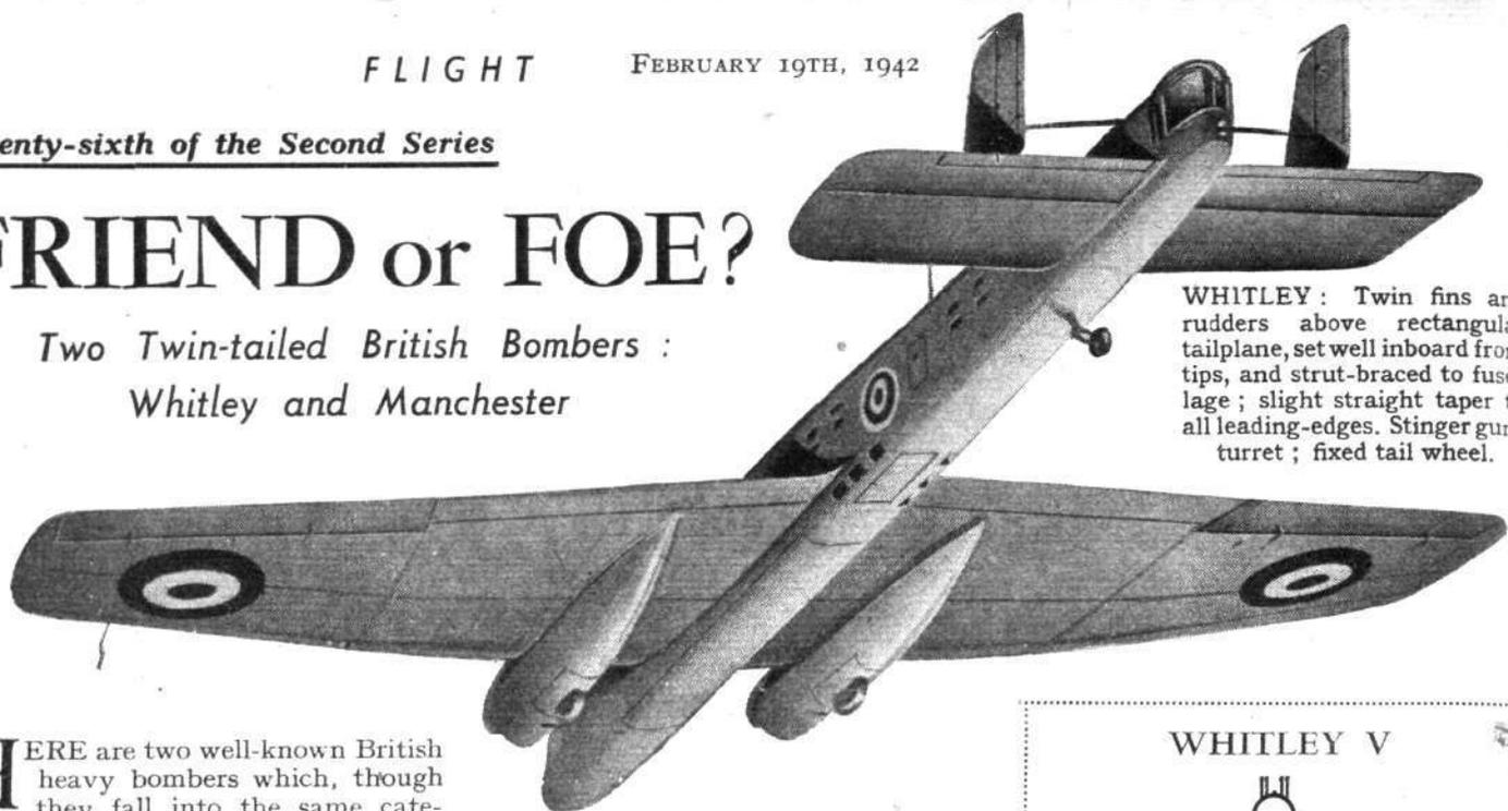
**WHITLEY :** Twin fins and rudders above rectangular tailplane, set well inboard from tips, and strut-braced to fuselage; slight straight taper to all leading-edges. Stinger gun-turret; fixed tail wheel.
