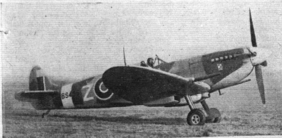
Three-quarter view of the improved Spitfire fitted with the R.-R. Merlin 61 engine and Rotol four-blade airscrew.
