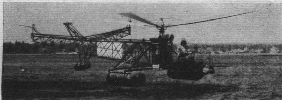
In its earlier stages the Sikorsky VS-300 had four rotors, a main lifting rotor and three control rotors. This was simplified later (as shown in the picture on the next page) into two, the main rotor and an airscrew at the stern for countering torque and for directional control.
