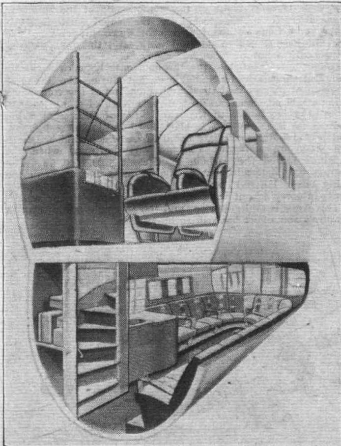
A spiral staircase joins the cocktail bar—observation lounge with the main cabin on the upper deck. Overall fuselage depth is 15ft. 9½in.
