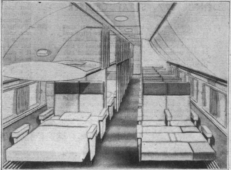
The upper berths in the main cabin are, during the day, apparently stowed behind arcuate segments of the ceiling. At left can be seen how lower berths are made up on the specially arranged seats.
