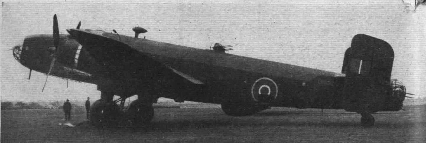
The blister on the belly of this Halifax is where the H2S scanner is housed. Usually, the rear end is Perspex although, as above, in some cases this does not apply.
