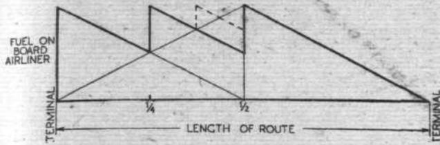
Fig. 2. Diagram showing that the optimum point of all refuellings should take place within the second quarter of the route distance.
