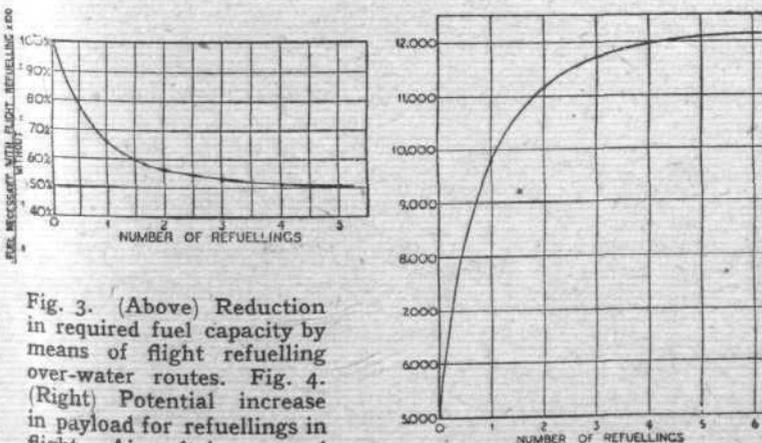
Fig. 3. (Above) Reduction in required fuel capacity by means of flight refuelling over-water routes. Fig. 4. (Right) Potential increase in payload for refuellings in flight. Aircraft is assumed to have 2,000 miles range, a normal payload of 5,000 lb. and a fuel consumption of one gallon per mile.
