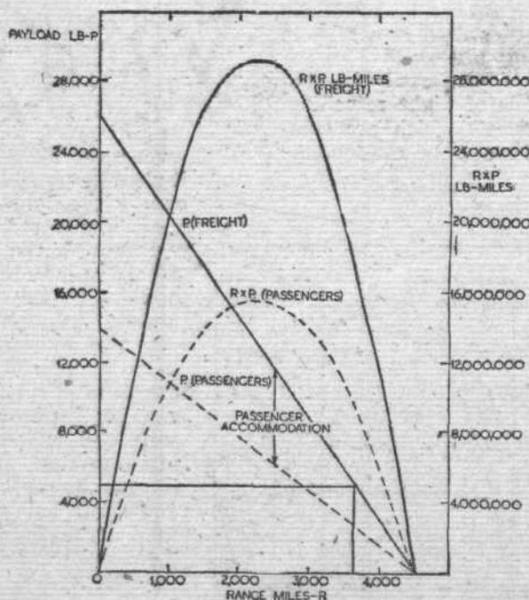
Fig. 5. Variation of freight load with range for given cruising conditions: if passengers are carried only, the broken line applies, if freight only, the full line, the difference being due to furnishings, galley equipment, etc.
