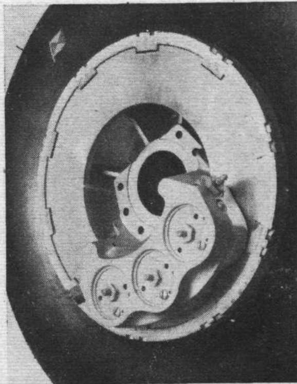
The Goodyear single-disc wheel brake. In the photograph is shown one type, with three hydraulic cylinders, while the sketch shows a single cylinder.
