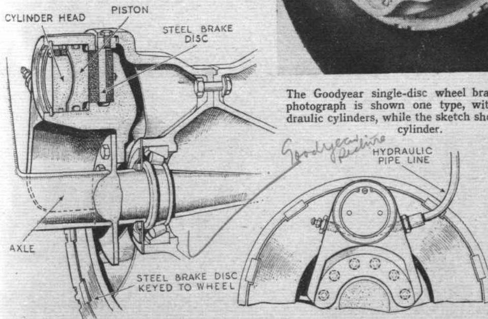
slightly, and hardened steel drive-keys are installed to accommodate the slots of the rotating steel disc.
