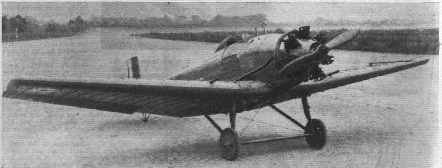
The 235 h.p. Lynx engined Vickers Vireo of 1928/29. It had many modern features, being an all-metal, cantilever monoplane with guns in the wings.
