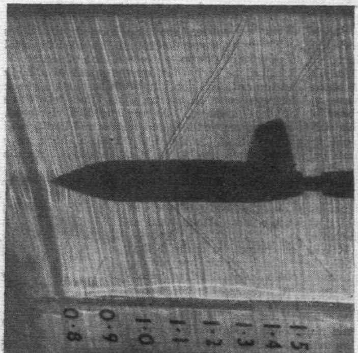
A model of the Miles M.52 during wind tunnel tests under conditions corresponding to 900 m.p.h. Shock waves are clearly visible.
