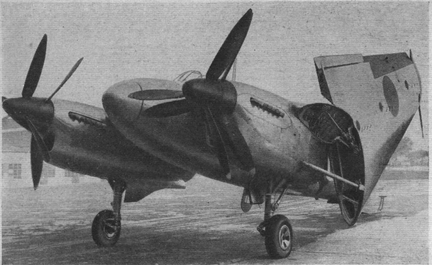
The remarkably neat wing folding arrangement of the Sturgeon can be appreciated here together with the close spacing of the nacelles and the necessity to swing the inner airscrew blades horizontal in order not to exceed a width of 20ft.
