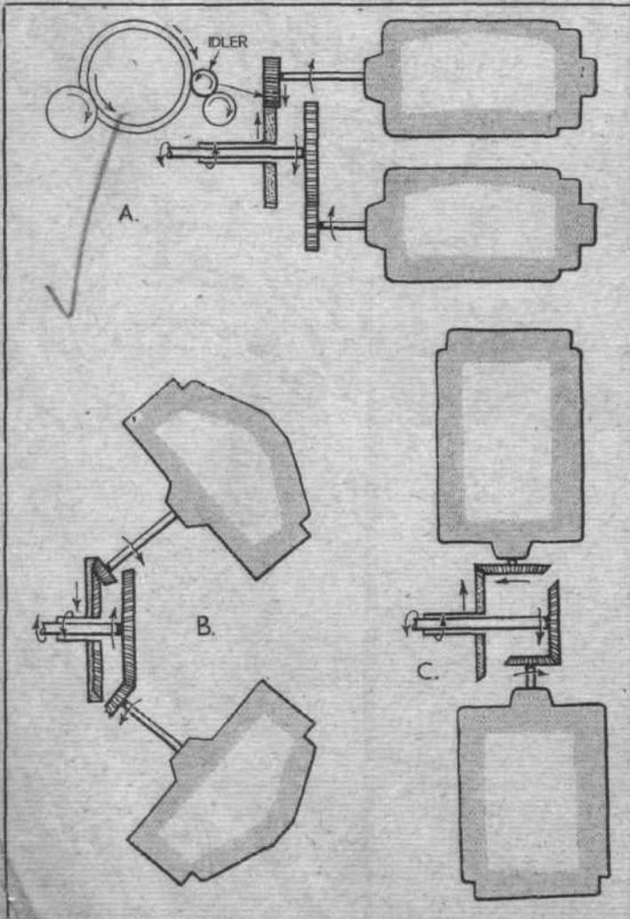
Three typical methods of driving coaxial airscrews. A: By parallel engines driving through spur reduction gears, one incorporating an idler pinion. B: By raked engines driving bevel reduction gears, one an internal type. This scheme is used for the Bristol 167. C: By opposed engines driving right-angle simple bevel reduction gears.
