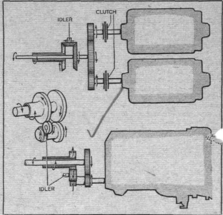
Two typical yet diverse methods of driving a contra-rotating airscrew. Top: By two parallel engines driving compound reduction gears through clutch couplings. Bottom: By one engine, as in Griffon and Merlin installations, where the crankshaft powers a double pinion and an idler is used to give contra-rotation.
