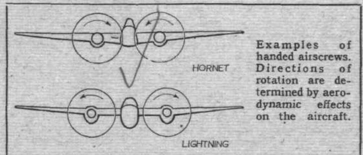
Examples of handed airscrews. Directions of rotation are determined by aerodynamic effects on the aircraft.
