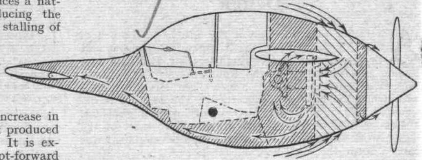
Diagrammatic section of fuselage showing location of noseplane, cabin, wings, engine and blower, and illustrating the airflow into the blower and out to the surfaces and propeller.
