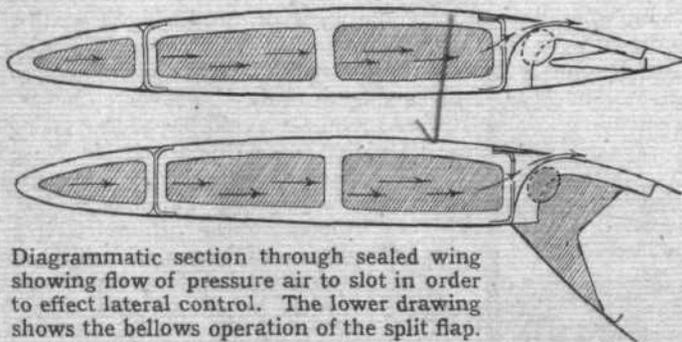
Diagrammatic section through sealed wing showing flow of pressure air to slot in order to effect lateral control. The lower drawing shows the bellows operation of the split flap.
