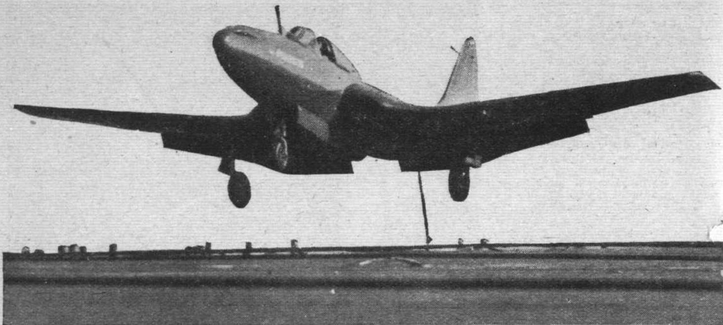
The first prototype of the McDonnell Phantom during deck-landing trials aboard U.S.S. *Franklin D. Roosevelt*.
