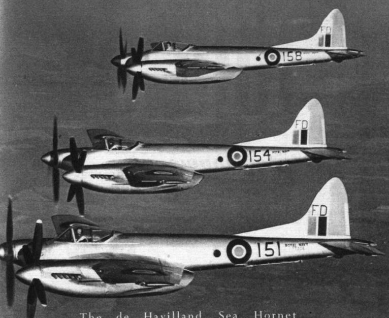
The de Havilland Sea Hornet (Rolls - Royce Merlin engines) is fitted with de Havilland handed constant-speed quick-pitch-change feathering propellers
