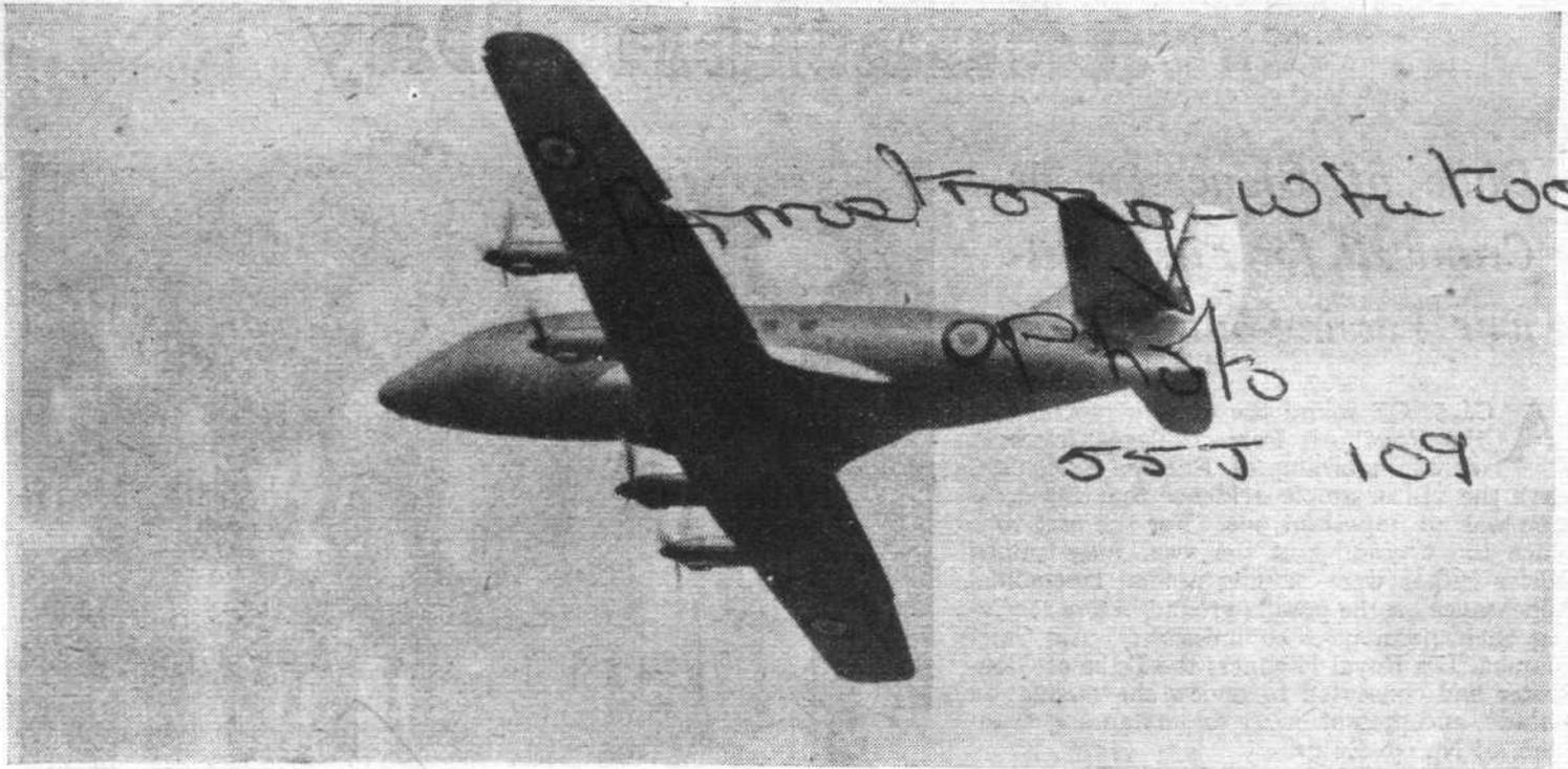
The first photograph to be taken of the A.W. Apollo in the air. Powered with four Mamba turboprops, it is designed to cruise at 305 m.p.h. at 20,000ft.
