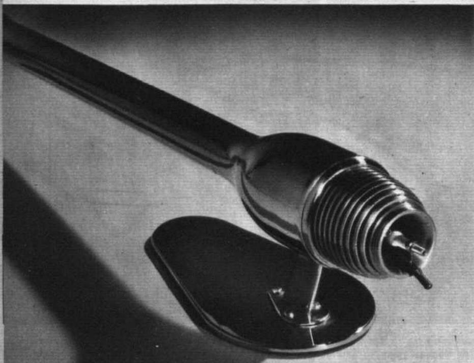
The Dyna-Jet unit is so compact that, dimensionally, it offers few installation problems. Starting air is provided by a tyre-pump or air bottle. Petrol is the fuel.
