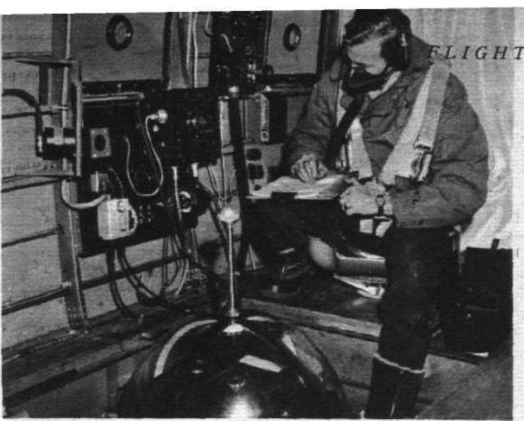
An operator in a Dakota with one of the new Williamson OSC-1 cameras. The transparent camera-enclosure is heated internally.
