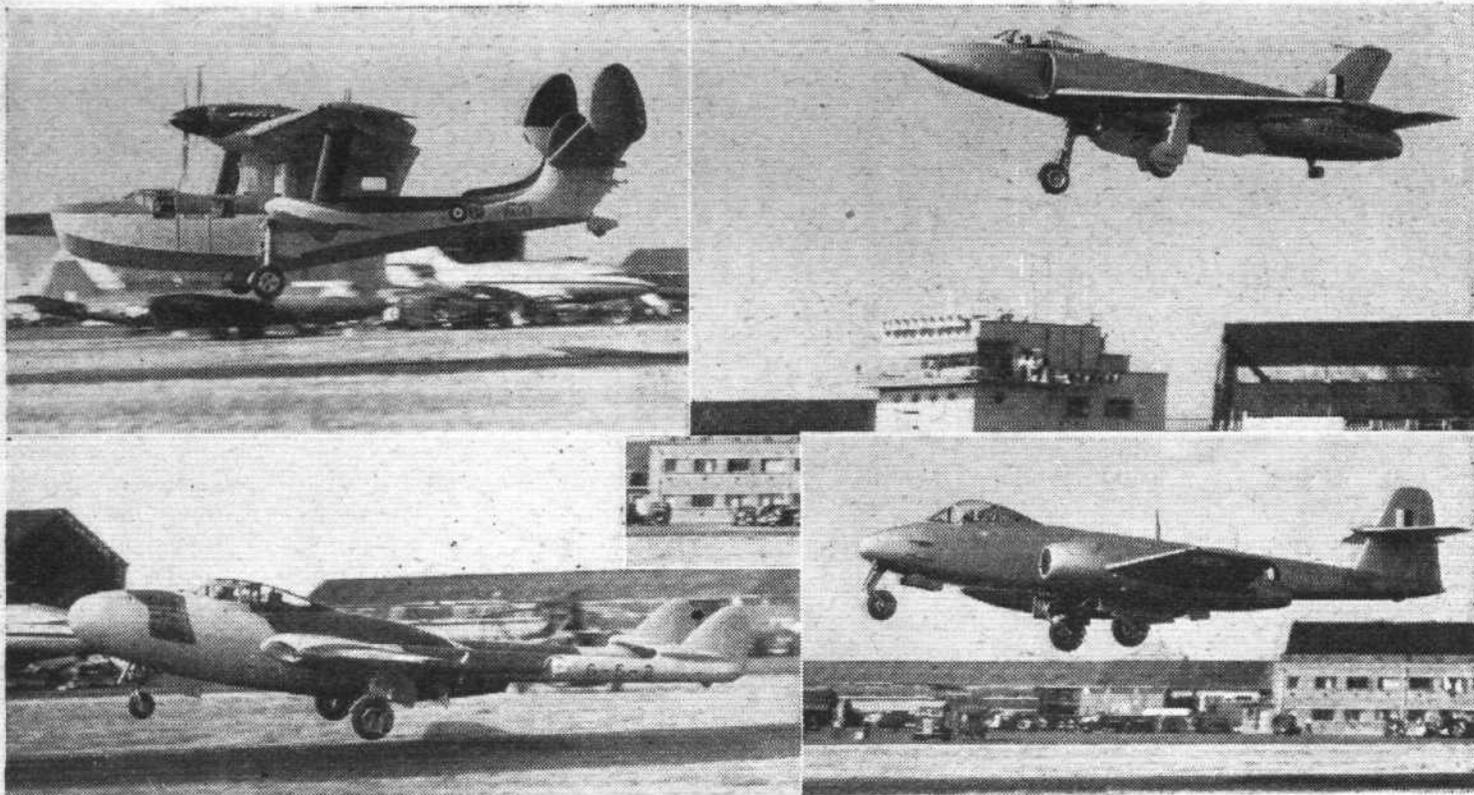
The Supermarine Seagull, seen at top left just before touch-down, now has dorsal and central fins. Likewise a Supermarine product, the Type 510 (top right) is, in its newest form, needle-nosed. Below (left) is the D.H.113 Vampire two-seater night fighter and (right) the latest Gloster Meteor variant—F. Mk.8, on which a new tailplane shape facilitates recognition from below.
