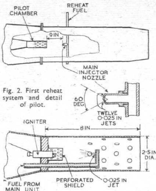
Fig. 2. First reheat system and detail of pilot.
