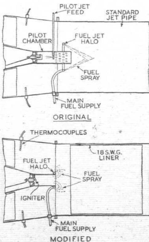
Fig. 3. Original and "halo" burners.
