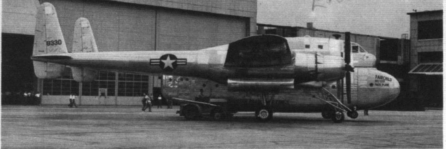
Military pack-mule: Specially designed for airborne logistics, the Fairchild XC-120 Pack-plane features a detachable cargo pod which can be quickly demounted and rolled away on its own undercarriage. The aircraft "sans pack" then flies away for another preloaded pack unit. Noteworthy is the quadricycle landing gear of the main aircraft.
