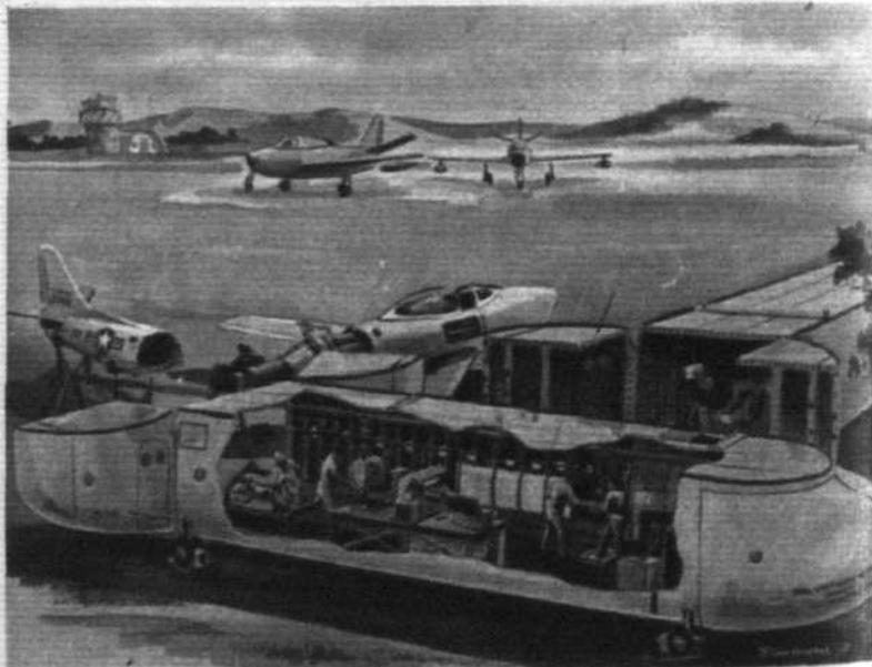
Making several round trips, one Pack-plane could bring into an airhead in a combat zone several packs filled with troops and supplies, leaving the pack units to be used as field hospitals, storage shelters, command posts, radar stations, repair shops, etc. Ambulance pods, carrying wounded, could be attached for the return trip.
