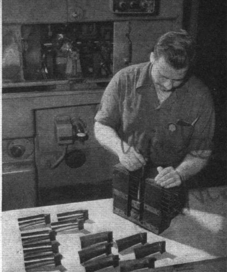
Checking blade-profiles, finished by the high-speed stropping process on the new machine seen in the background. In the foreground is a batch of blades awaiting finishing.
