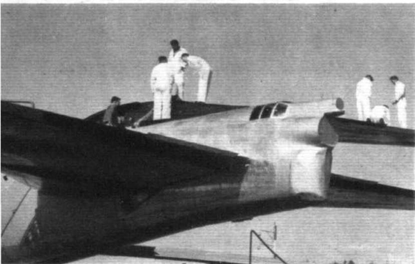
Incomplete tail-gun emplacement of the Boeing B-52 Stratofortress—the world's largest bomber. (Intended armament is four 20 mm guns.)
