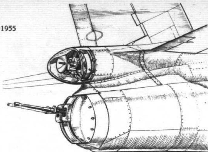
General Electric tail turret, with two 20 mm guns, on Boeing B-47. (Search-radar housing shown sectioned.)
