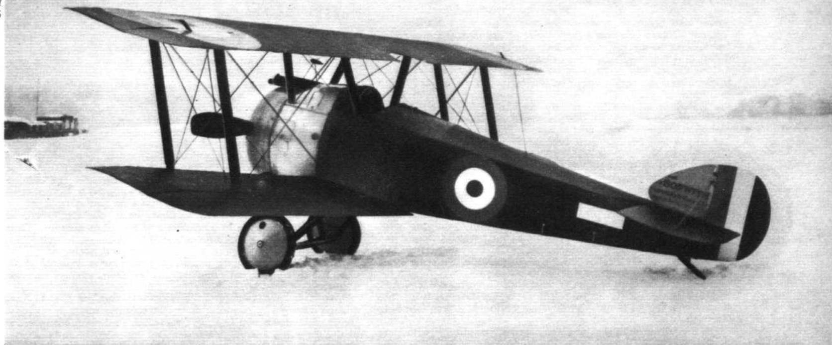
In the snow at Brooklands, early in 1917, is seen the first Camel of all, an F.1, with 110 h.p. Clerget rotary engine.
