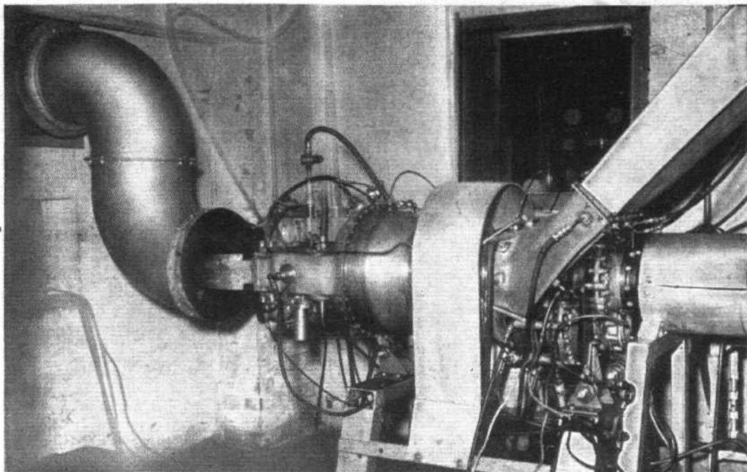
A Blackburn-Turboméca Turmo 600 undergoing endurance testing. The output gearbox is partially hidden by the sloping exhaust duct, and the dynamometer brake is off to the right (see drawing on p. 756).
