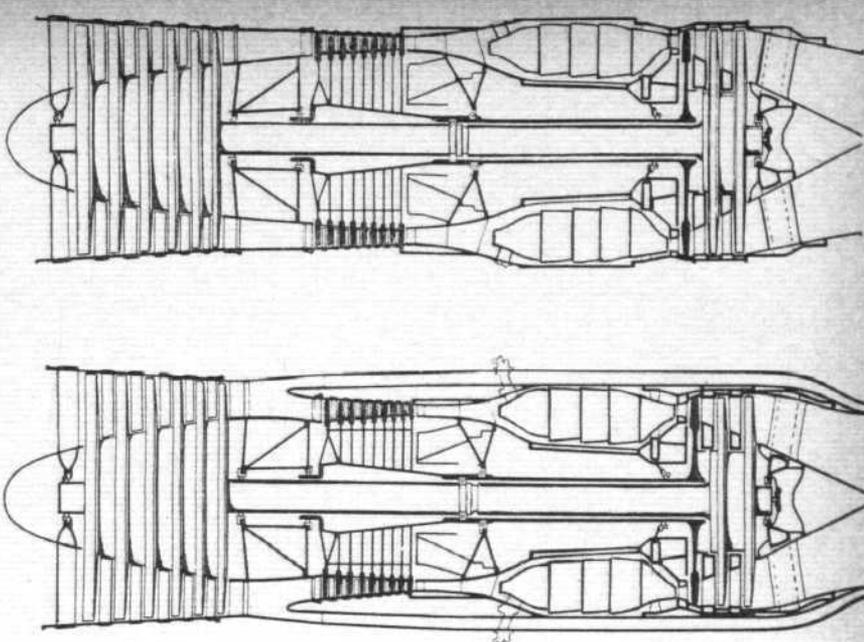
These two sectional elevations, illustrating the essential differences in the layout of turbojets of the plain (top) and by-pass types, were among the illustrations accompanying Mr. Lombard's paper.
