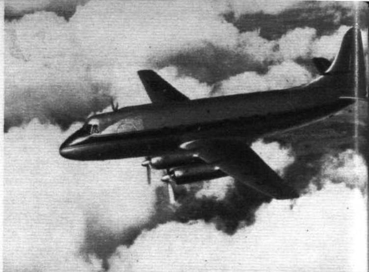
Prototype V.630 in the original colour-scheme. At 40,000 lb (later 43,000 lb) the aircraft was 20,000 lb lighter than today's Viscounts.
