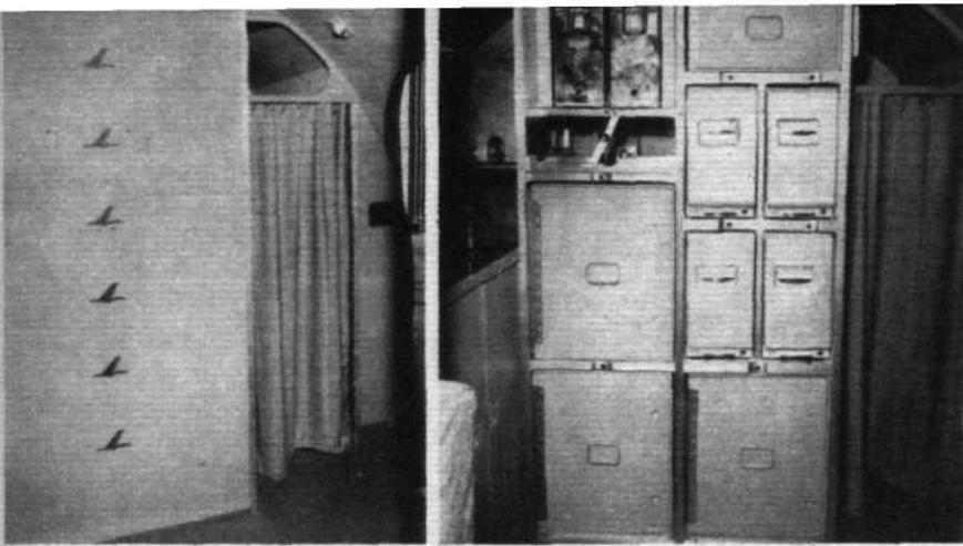
When not in use, the very compact galley of the V.744/5 is hidden from sight by a neat roller blind (left). At right is shown the pantry and sink. The steward's station also incorporates a control panel.
