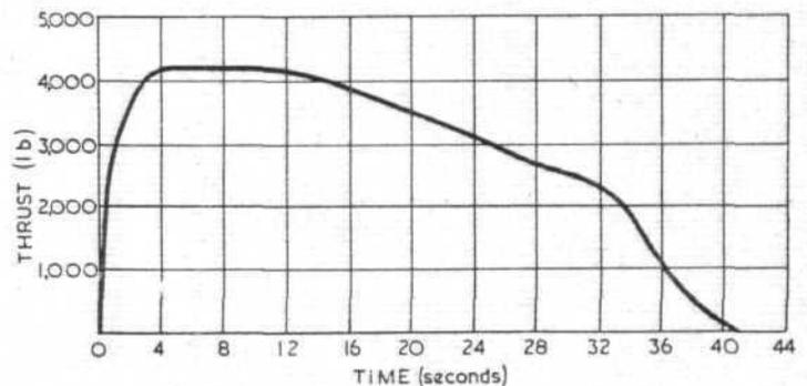
Thrust plotted against time for typical Super Sprite operation.
