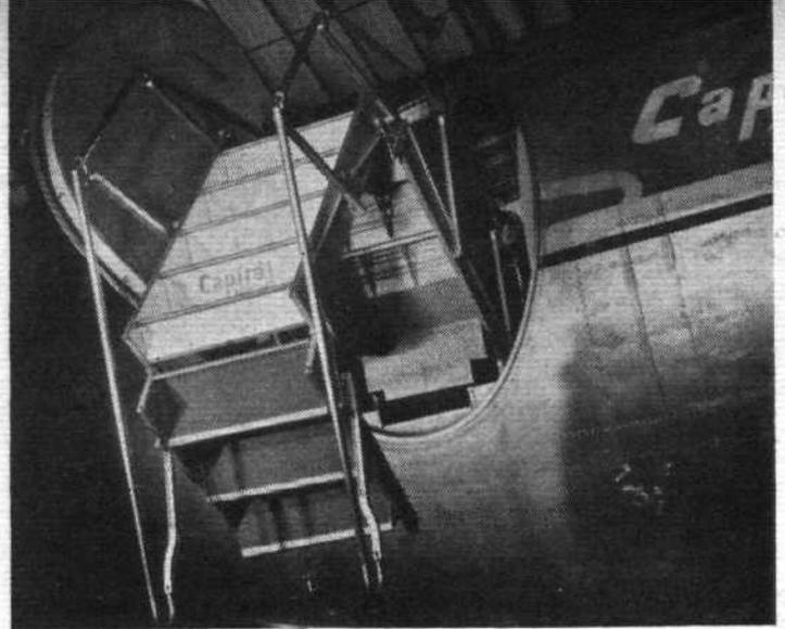
**INSTEPS:** Built-in passenger steps—seen above in a Vickers test rig—are to be fitted to the majority of the Viscounts on order for Capital Airlines. Hydraulically operated, they will be offered as standard on aircraft for the American market. Installation is in the forward door and the weight penalty is in the region of 260 lb.
