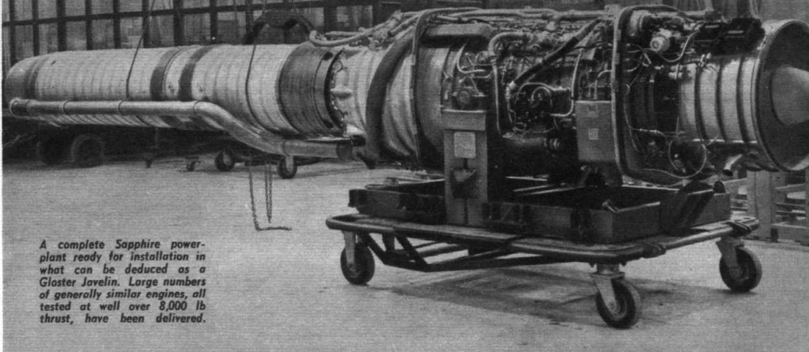
A complete Sapphire power-plant ready for installation in what can be deduced as a Gloster Javelin. Large numbers of generally similar engines, all tested at well over 8,000 lb thrust, have been delivered.
