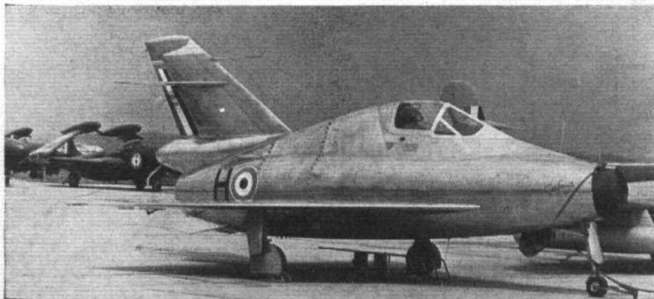
Area ruling? The Gerfaut at Le Bourget last year with a large tail blister, two rows of vortex generators round the fuselage and supplementary under-fins. (Right) Gerfaut II? The model on the S.N.C.A.N. stand at the 1955 Paris Salon. The size of the jet orifice is most marked, suggesting an advanced form of afterburning. The wing-tip shape is different from that of the Gerfaut I and the ailerons are not inset.
