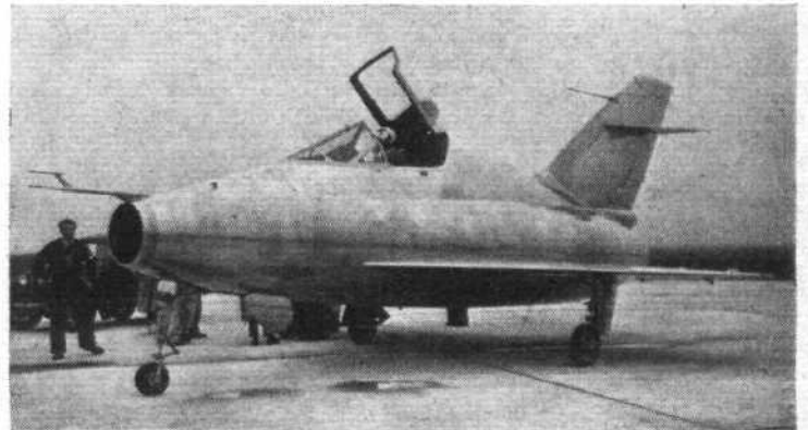
The S.F.E.C.M.A.S. Ars.1301 glider just before final flight-testing with its nose-plane fitted and its tail-plane retained as a precautionary measure. (Below) The S.F.E.C.M.A.S. 1402 (later named Gerfaut) at the time of its first taxiing trials in late 1953.
